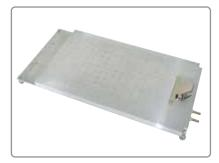
Elcometer 4900 free standing vacuum tables provide an ideal surface for manual application of films on test charts or samples. Made of perforated aluminium, the Elcometer 4900 keeps a wide range of test pieces absolutely flat ( $2.3\mu$ m variation over a 100mm length), including glass, plastic sheets, contrast charts, etc., ideal for thicker, more substantial test pieces.
