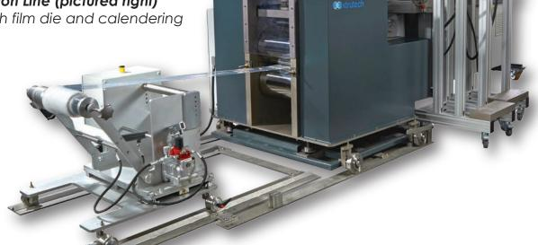
The XTS35 is a versatile extruder that can serve both laboratory and production functions. The 35mm is ideally used as a lab machine when higher free volume is necessary. It is also perfect for low-scale production and offers a high throughput particularly for specialty products.
